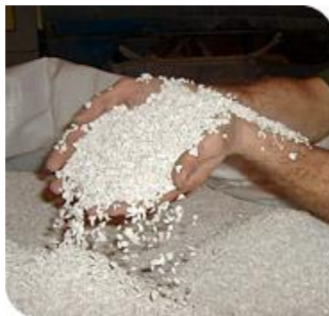
5. Once the waste has been washed and all impurities removed, it is then processed to the pellet form.
